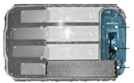
Power electronics combination module (OBC and DC-DC converter)
